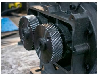
CP Series blower internal helical gears.
