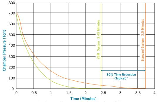
Data from actual laboratory testing from atmosphere to 0.1 Torr. \* Actual time savings will vary depending on system staging ratio and chamber volume.
