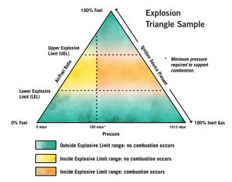
The blower or booster is intended to internally handle explosive gas mixtures up to the critical gas combustion pressure of approximately 100 mbar. This pressure varies by gas type. All product selections are required to be evaluated through Tuthill's VBXpert Portal sizing software prior to quotation. For pressures greater than 100 mbar ATEX Internal classification is not supported.
