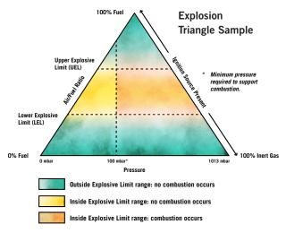
The blower or booster is intended to internally handle explosive gas mixtures up to the critical gas combustion pressure of approximately 100 mbar. This pressure varies by gas type. All product selections are required to be evaluated through MD-Kinney's VBXpert Portal sizing software prior to quotation. For pressures greater than 100 mbar ATEX Internal classification is not supported.
